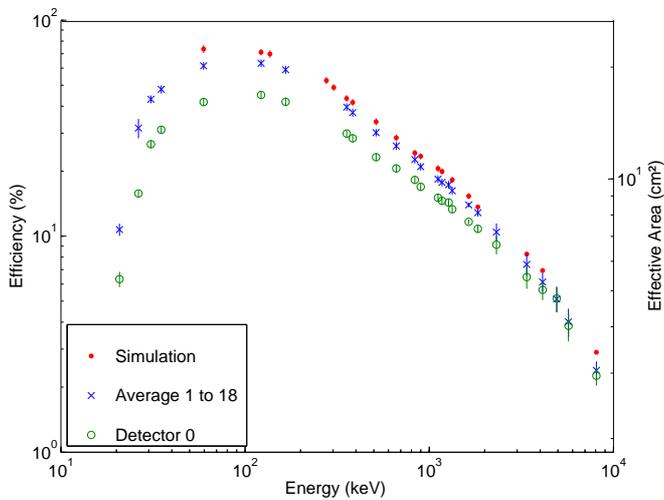
**Fig. 2.** Full-energy peak efficiency for sources on the SPI optical axis ( $\alpha = 0^\circ$ ), without mask. An average for detectors 1 to 18 is shown; detector 0 is plotted separately (see Sec. 5.2). The measurements are compared to Monte-Carlo simulations.
