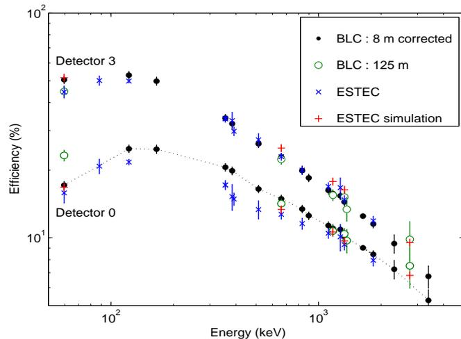
**Fig. 5.** The on-axis, full-energy peak efficiencies of detector 0 and 3 for SPI with its mask. The data are: 8 m BLC data without mask corrected for the mask absorption ( $\cdot$ ), 125 m BLC data with mask, ( $\circ$ ) and 8 m ESTEC data with mask ( $\times$ ). For detector 0, the disagreement between the curves shows the difficulty of alignment device modelisation.
