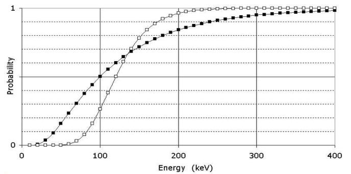
**Fig. 10.** For  $\text{PMT}_1$  (solid),  $E_{\text{th}} = 100\text{ keV}$  and  $a = \sqrt{50}$ , for  $\text{PMT}_2$  (open),  $120\text{ keV}$  and  $\sqrt{10}$ . These curves illustrate the large differences between ACS crystals and PMTs combinations.
