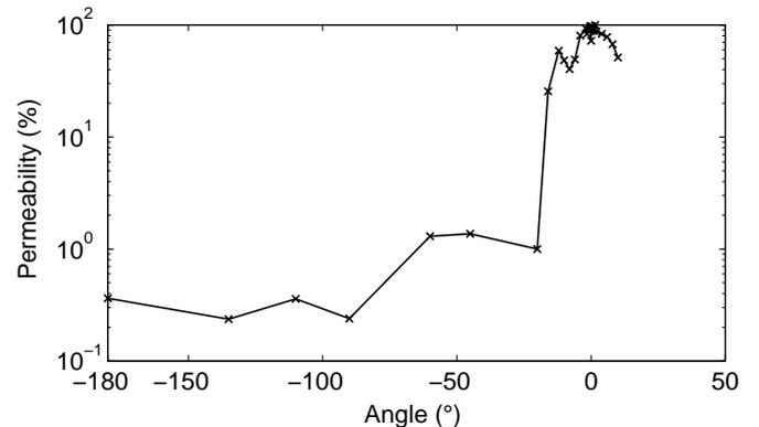
**Fig. 11.** ACS permeability as a function of the angle from the axis (BLC,  $^{137}\text{Cs}$  source)
