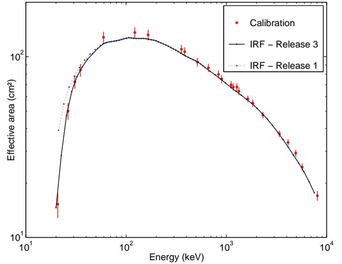
**Fig. 6.** Full-energy peak effective area of SPI telescope using all events (SE+ME). This curve is representative of the in flight effective area for an on-axis source. We compare it to the response matrix before the launch (release 1, nov 2002) and after the launch (release 3, july 2003).
