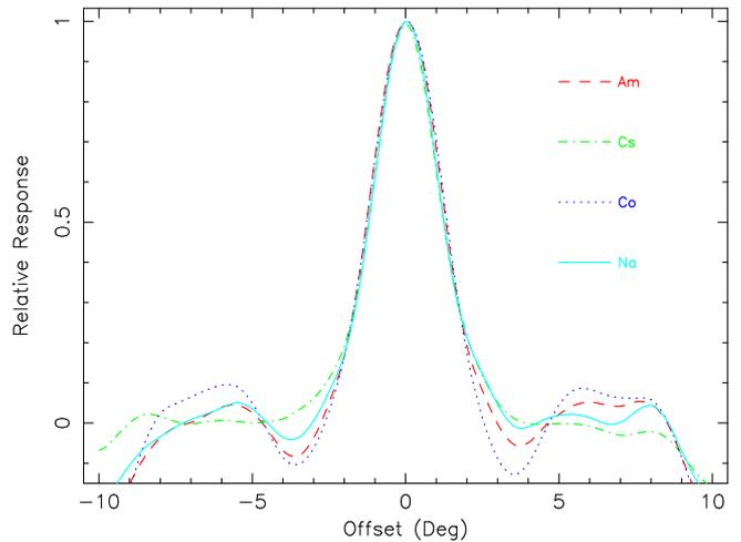
**Fig. 7.** The PSF determined from measurements of 4 different sources at 125 m. Each curve is the mean of cross-sections through the response in two orthogonal directions; a background level has been subtracted from each and the curves normalized to the same peak height. The mean FWHM is  $2.55^\circ$ . ( $^{241}\text{Am}$ : 60 keV;  $^{137}\text{Cs}$ : 662 keV;  $^{60}\text{Co}$ : 1332 keV;  $^{24}\text{Na}$ : 2754 keV)
